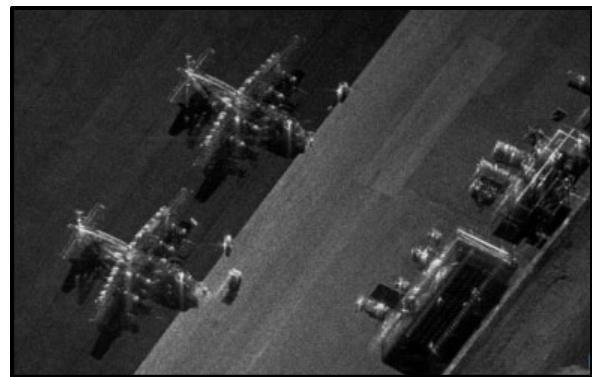
Figure 2-2-3: Ka-band RADAR image: C-130s on flight line at Kirtland AFB. (Photo: Sandia National Laboratories, Airborne ISR)
